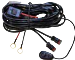
Part No. 270441 CABLE KIT 12-24V 2 pcs DT-connectors females/plugs. With on/off switch. Max 2x 100W @ 12V, 2x 100W @ 24V.
