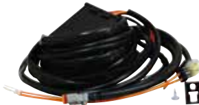
Part No. 270413 CABLE KIT PROFESSIONAL 12-24V 1 pcs DT-connection female/plug or 3 pcs cable-connectors Includes: Wires, relay, line fuse. Max 216W @ 12V, 288W @ 24V.
