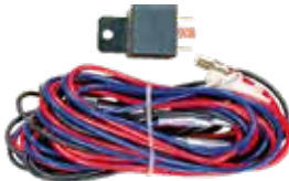
Part No. 270415 CABLE KIT 12V For two driving lights | Includes: Wires, relay, line fuse. Max 2x 240W @ 12V.
