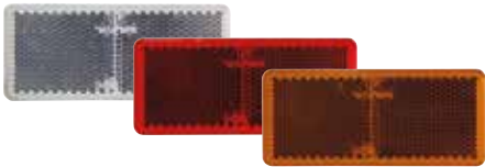
Part No. 810659-4 white 810660-4 red 810661-4 amber REFLECTOR Measurments: 96x42mm | With tape | CC: 70mm | E-approved according to regulation: ECE R3 | Packed in 4 pcs/pack
