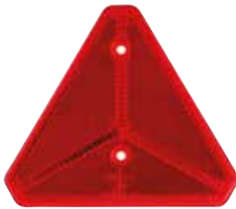
Part No. 810637 REFLECTOR Measurments: 143x125mm | With screw holes | CC: 70mm | E-approved according to regulation: ECE R3
